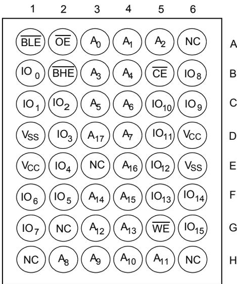
Figure 2. 48-Ball VFBGA (Pinout 2) <sup>[2, 3]</sup>
