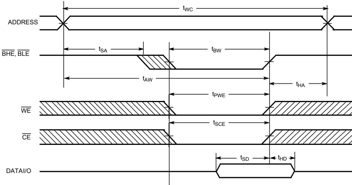
Figure 8. Write Cycle No. 3 ( $\overline{\text{WE}}$  Controlled,  $\overline{\text{OE}}$  HIGH During Write)<sup>[19, 20]</sup>
